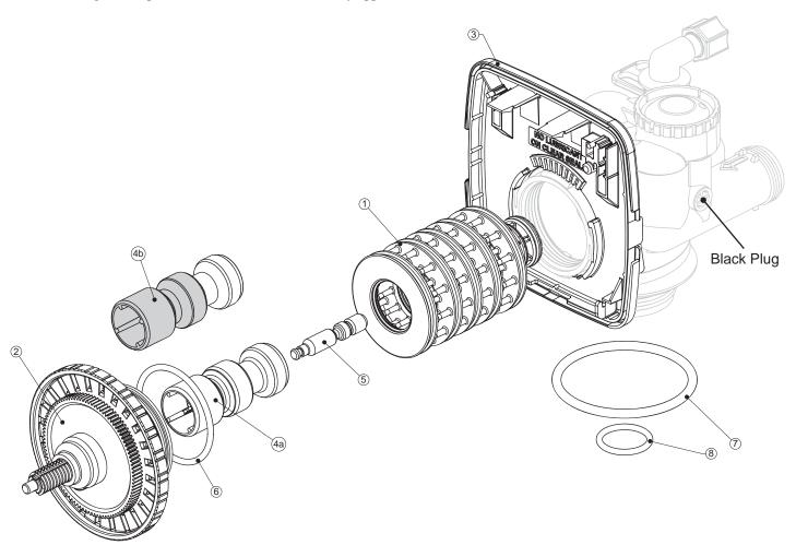
WS1.25 Drive Cap Assembly, Downflow Piston, Regenerant Piston and Spacer Stack Assembly
